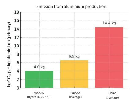
Carbon emissions per kg of primary aluminium depending on production location. A comparison between ErgoSafe's choice of Hydro REDUXA in Sweden and the average emissions from aluminium production in Europe and China. Hydro REDUXA is produced using hydropower and has approximately 4 kg CO<sub>2</sub> per kg. Europe's primary aluminium averages around 6-7 kg per kg (2023 data), while China is around 14 kg per kg.
